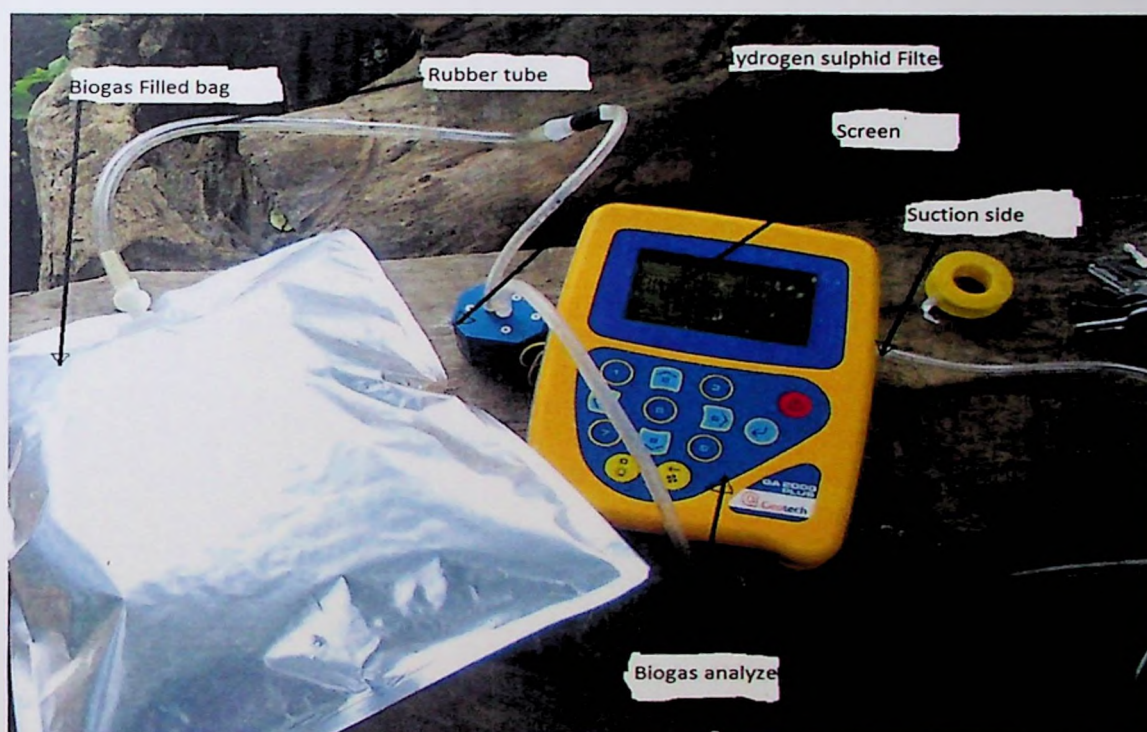
Figure 3.2: Biogas Analyzer setup
