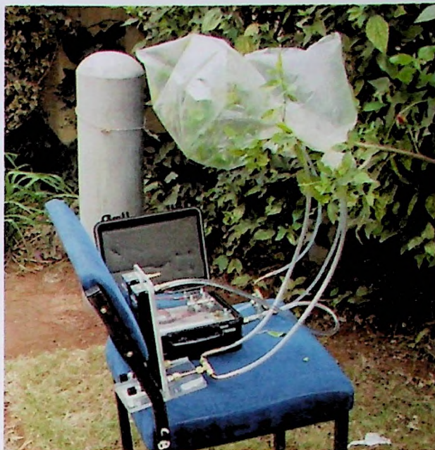
Figure 6.2 A battery powered pump used for trapping volatiles in the field
