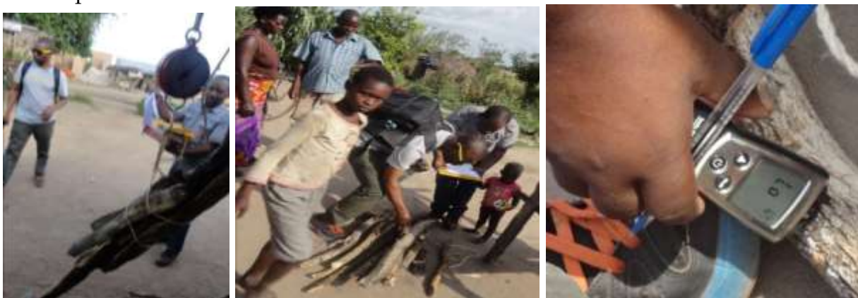
Figure 13: Measuring household fuel consumption in Nakitoma, Nakasongola district; Left-Fuel weighing on a spring balance during KPT; Middle-Determination of moisture content; Right-Moisture meter (Protimeter Mini BLD2000)
